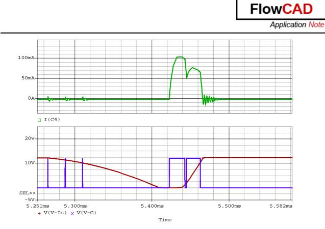
In the above diagram you can see how C4 will be charged while M1 switches on.
