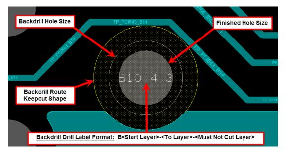
Backdrill locations clearly identified with special drill labels and hollow circle showing the backdrill diameter
